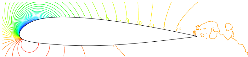
Figure 13: Instantaneous resolved pressure on the Chalmers mesh when wall functions are used (Comp. # 4).
