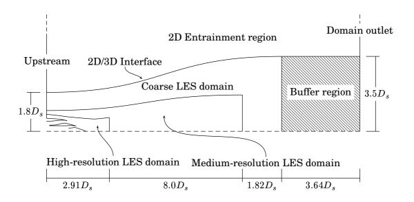
Figure 4.6: Computational set-up – dual-stream jet.  $D_s$  is the secondary stream nozzle outlet diameter ( $D_s = 0.275[m]$ ).
