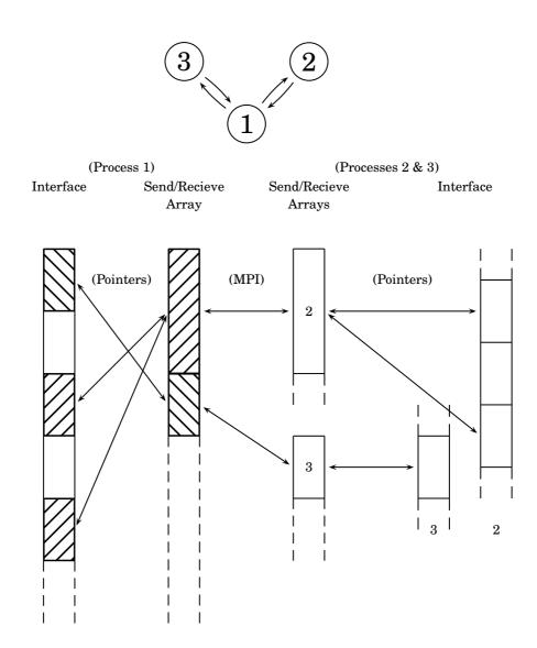
Figure C.1: Send and receive structures. A schematic illustration of the MPI communication between three processes with common mesh block interface areas.
