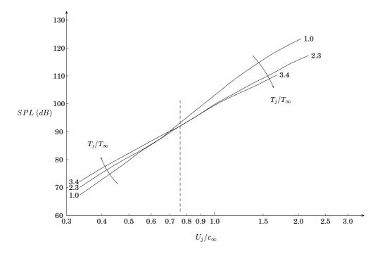
Figure 5.1: Sound pressure levels as a function of jet Mach number for different jet to ambient temperature ratios at  $\theta = 90^{\circ}$  ( $\theta$  being the angle from the x-axis). Measurements by Tanna (1977).
