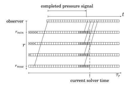
Figure 4.10: The upper row of cells represents the observer pressure signal and the lower ones the time series of sound source parameters for four surface or volume elements.  $\tau_r$  denotes retarded time.
