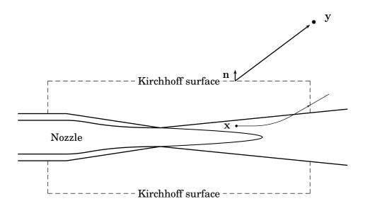
Figure 3.2: Sound generated in the shear-layer location, x, is propagated in the Navier-Stokes solver and extracted from the Kirchhoff surface to the far-field observer, y. The surface is open in the downstream end to prevent it from entering the hydrodynamic jet region.
