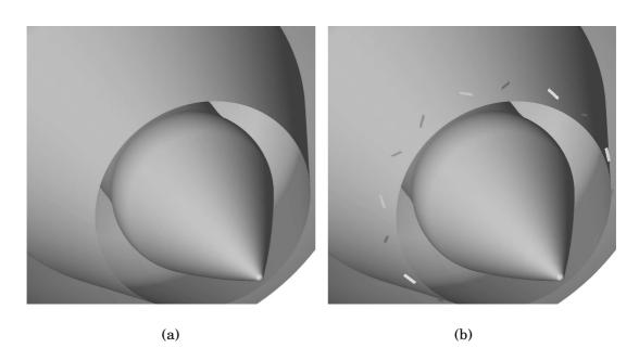
Figure 6.1: The CoJeN coaxial nozzle base configuration (a) and with the application of vortex generators (b)
