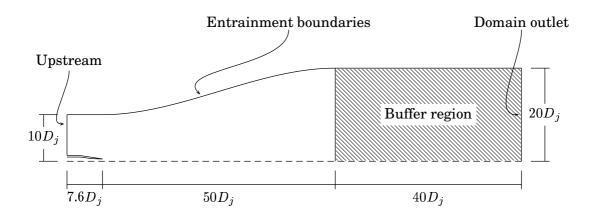
Figure 4.5: Computational set-up – single-stream jet.  $D_j$  is the nozzle outlet diameter ( $D_j = 0.05[m]$ ).
