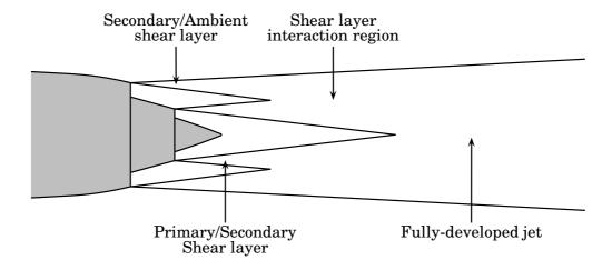
Figure 5.2: Flow regions in a developing dual-stream jet
