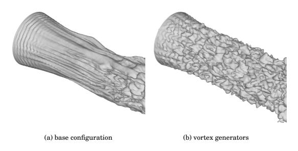
Figure 6.2: The primary shear layer in the near-nozzle region visualized by density iso-surfaces
