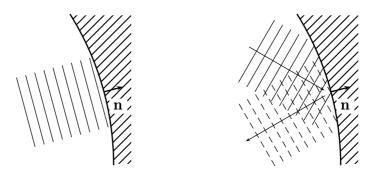
Figure 4.7: A plane wave reaching the boundary with the transport direction aligned with the surface normal is perfectly absorbed (left), whereas a wave not aligned will be partly reflected (right).
