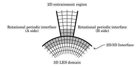
Figure 4.9: Interface between the 3D LES domain and the "2D" entrainment region in the dual-stream jet computational set-up.
