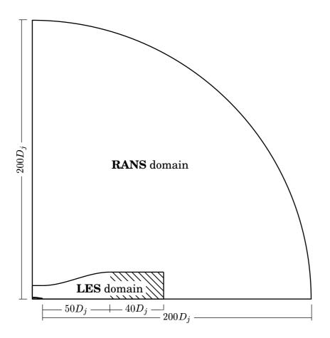
Figure 4.8: Computational domains for the LES and the RANS calculations of the single-stream jet
