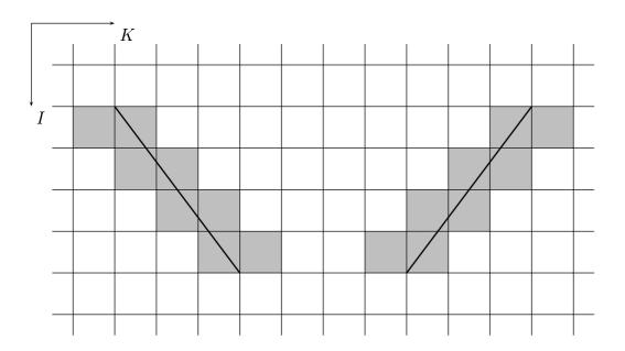
Figure 6.4: Schematic illustration of a vortex generator pair (cf. Figure (6.1(b))). Volume forces are distributed to the two cells closest to the vortex generators in each row in the local K-direction (highlighted cells).
