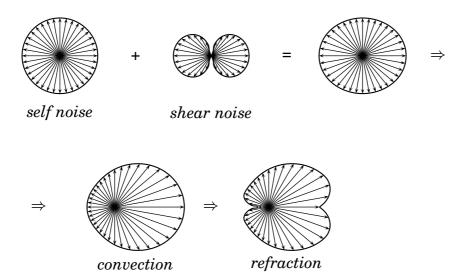
Figure 1.3: Superimposition of the noise generated by the turbulence itself, self noise, and the noise generated by interaction of the mean shear flow and turbulence, shear noise, gives the upper right sound pattern. Convection and refraction affect the pattern of radiated sound, and the result is the directional sound pattern in the lower right figure.
