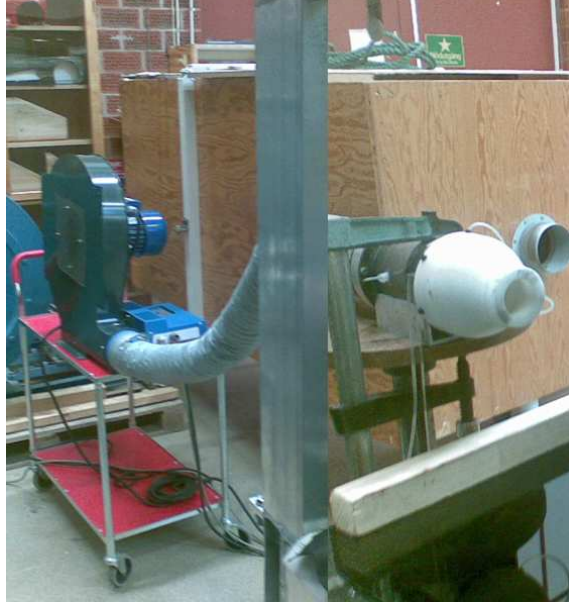
Figure 2: The air jet generator used in the calibration procedure.
