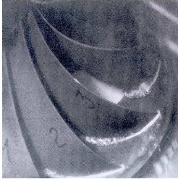
Figure 4.15: Photograph of the inlet edge cavitation development at the best efficiency operating point. Picture taken from the GAMM Proceedings.
