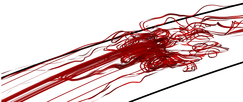
Figure 16: 3D view of streamlines showing the transitional separation bubble.
