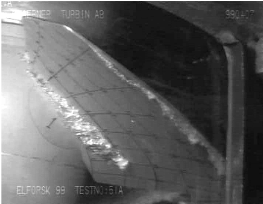
Figure 1.6: Hub and tip clearance cavitation. The picture shows the suction side of a Kaplan runner blade. The leading edge is at the upper left and the trailing edge is at the lower right. The hub is to the left. The cloudy structure close to the hub and the streaky structure close to the blade tip are cavitation bubbles that have developed in low static pressure regions. Picture courtesy of M.Grekula and G.Bark, Department of Naval Architecture and Ocean Engineering, Division of Hydromechanics, Chalmers University of Technology.
