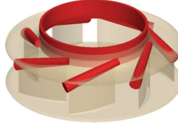
Figure 3. Mesh refinement regions (red) at the inlet gap and blades top region.
