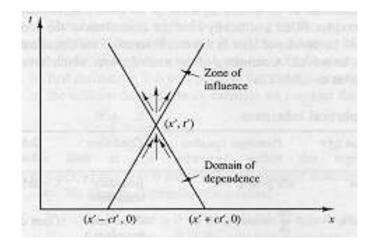
The propagation of disturbances to a point P for hyperbolic, parabolic and elliptic equations are summarized in the figure below (fig. 2.10)
