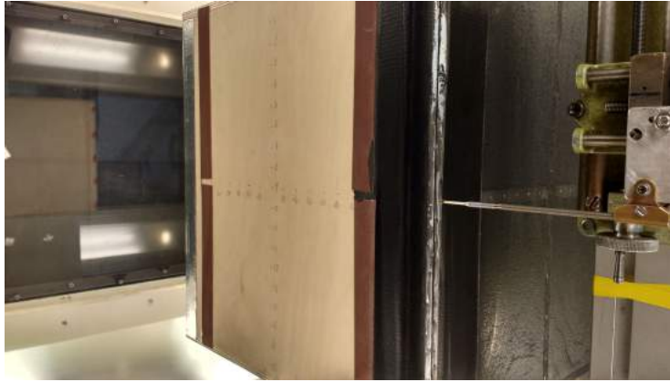
Figure 2.8: The hot wire anemometry setup
